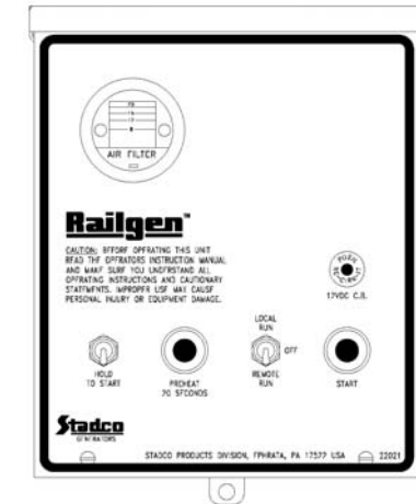
Unit Mounted Panel: 10.3"W x 8.3"H
